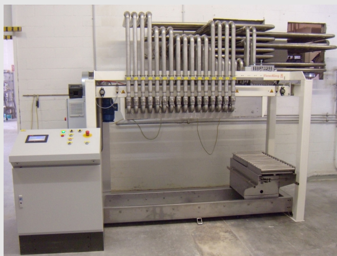
Gravimetric filling installation for 32 components by means of a moveable scale. All components connected by piping to fixed tanks and exchangeable IBC containers.
